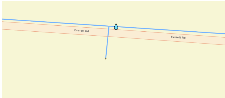
Figure 5: Example of leak found near the corporation on a water main. In this case, the leak sound will be loudest on the customer meter closest to the leak.
